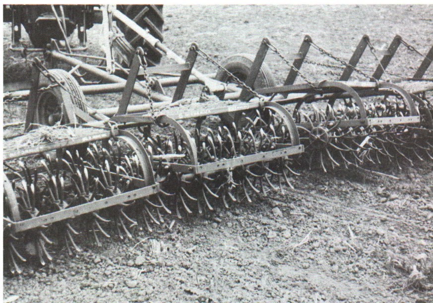
Figure 8—The rotary hoe is effective only when used at high speeds on relatively dry soil. Both dry bean and soybean producers have liked this implement because it tears out small weeds and destroys thin crusts. Some feel that this tool is not as effective as in the past. The successful use of herbicides reduced the need for this tillage tool.
