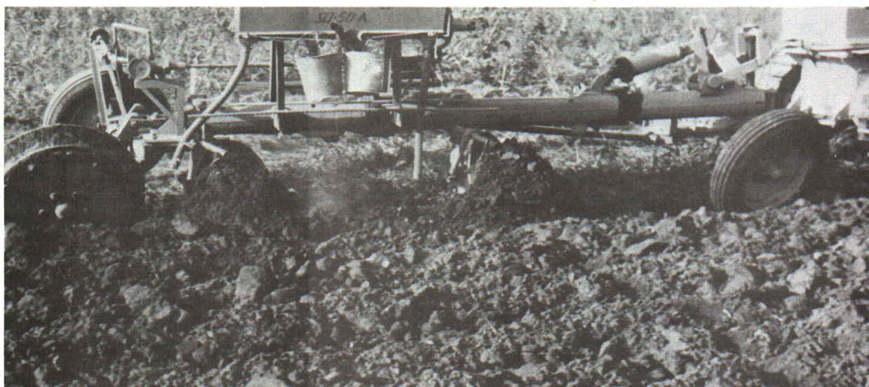
Figure 4—Giant disc plow used in Michigan research program. Penetration to 30 inches was possible. This plow was modified for application of fertilizer and lime as plow down treatments. While this plow was designed with four discs, only two were used because of inadequate power. Deep plowing is the only known way of improving the soil conditions described in Figure 1.
