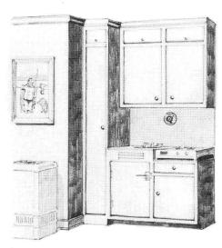
2. View into the kitchen area shows a broom closet, cupboards above and below counter, a mechanical or ice refrigerator, and a hot plate, located at convenient working height. If preferred, these items can be purchased as one manufactured unit and installed in the same amount of space.
