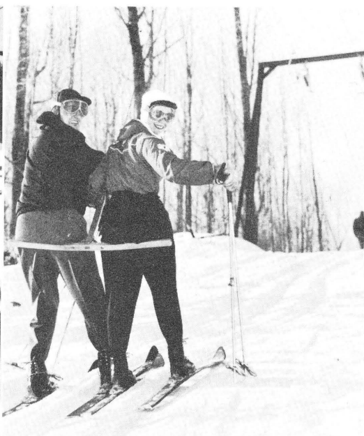
Fig. 12. T-bar. A durable type which takes up two at a time. T-bars can be replaced with chairs.
