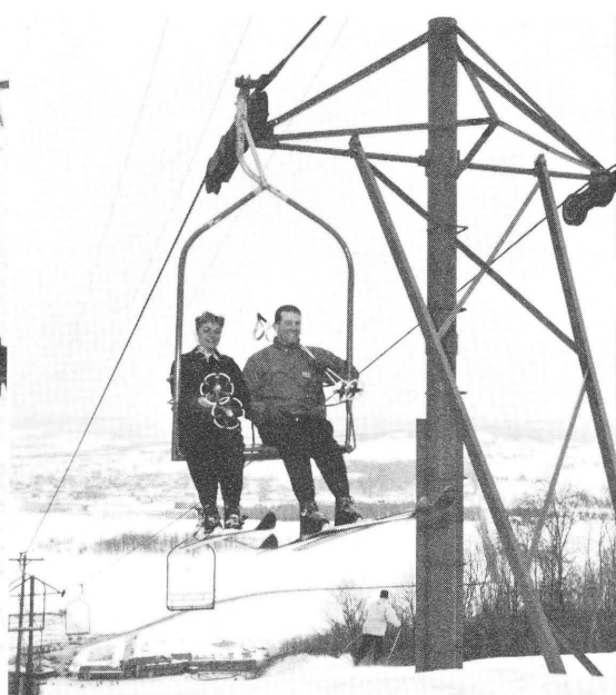
Fig. 13. Chair Lift. Deluxe uphill equipment, best suited to long and steep slopes.
