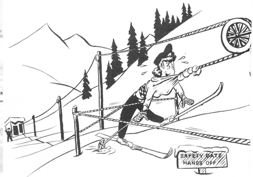
Fig. 10. A positive power cut-off device is an absolute necessity for all rope tows. Ample area for landing ahead of safety cut-off is needed.
