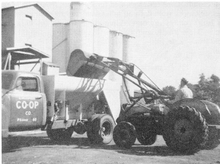
Fig. 1. This type of equipment is commonly used to load and spread bulk fertilizer. The spreading width is usually from 20 to 25 feet.
