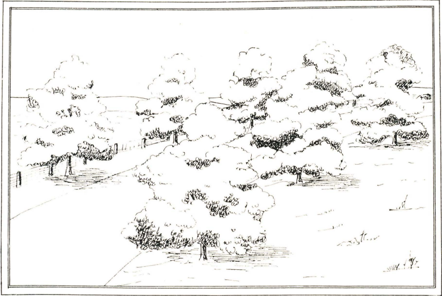
Fig. 12.—Trees planted along highways traversing a naturalistic landscape should not be disposed in definite rows.
