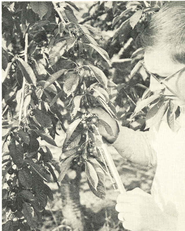
Fig. 1. The force to detach cherries was measured periodically during the season.
