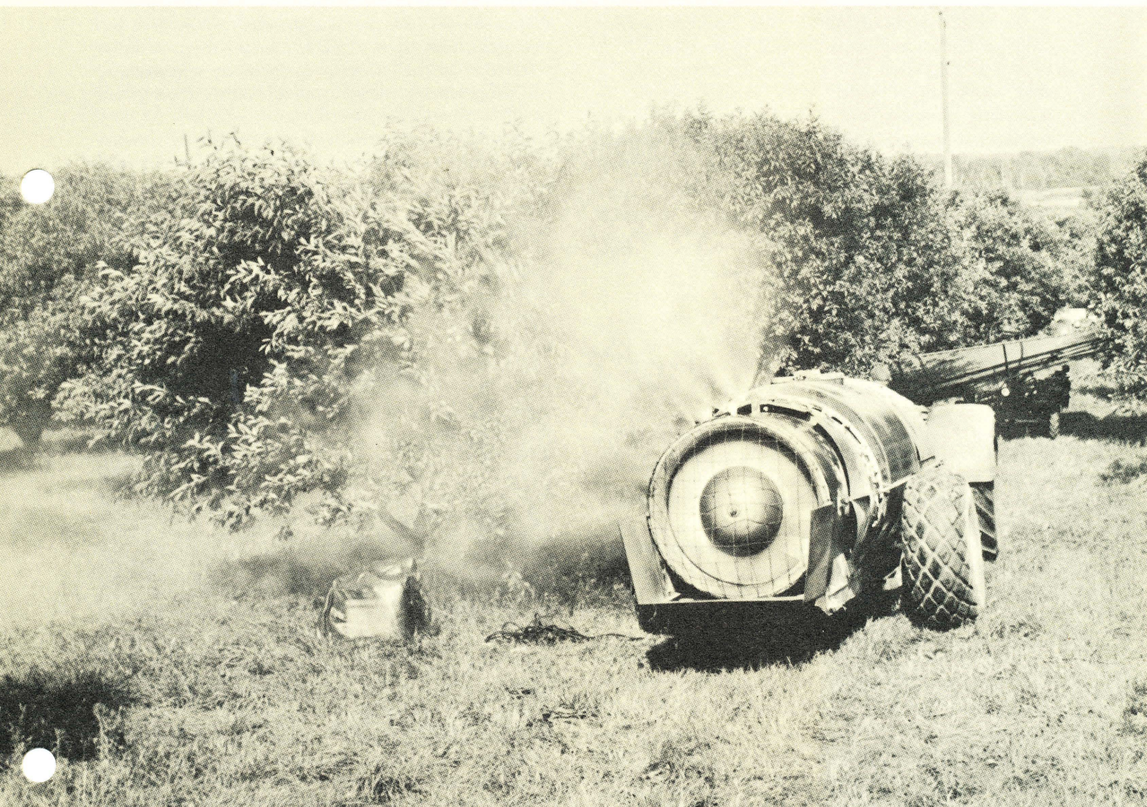
Preharvest spray cooling of tart cherries using an orchard air blast sprayer
