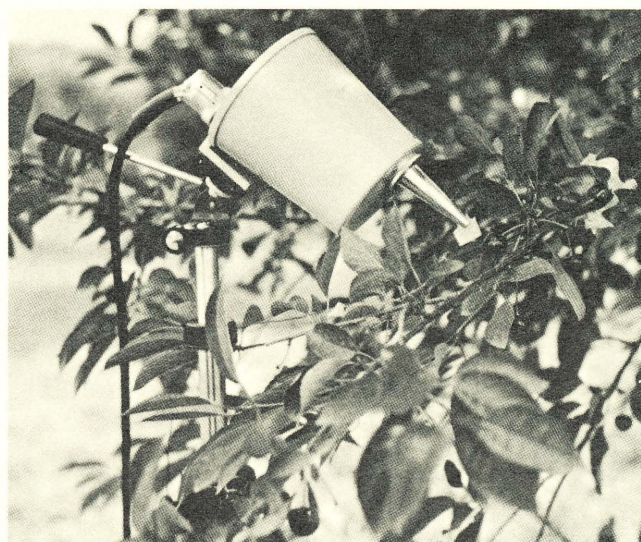
Fig. 1. Measurement of cherry temperature: surface —infrared non-contact thermometer; internal — thermocouple inserted in cherry (held by masking tape).
