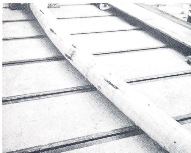
Fig. 10. Typical failure in red pine pole.
