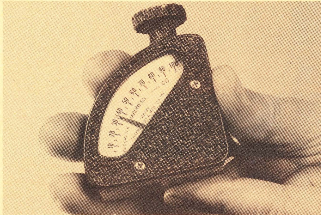
Fig. 2. The Durometer used to measure red tart cherry fruit firmness. As indenter is depressed a reading is obtained. Reading must be taken while indenter is depressed.
