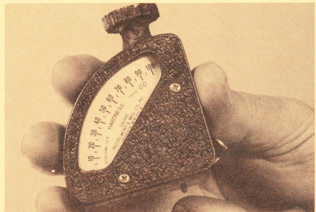
Fig. 1. The Durometer, Type 00, is used to measure red tart cherry fruit firmness. Indenter at bottom is 3/32 in. in diameter with spherical point; 100 on the scale equals 4 oz.
