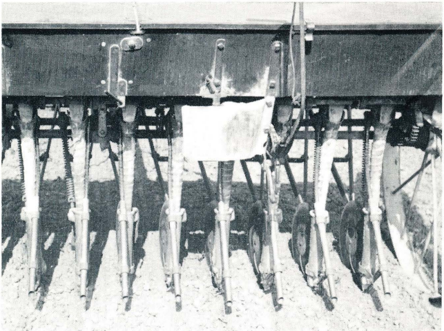
Standard model grain drill adapted for band seeding
