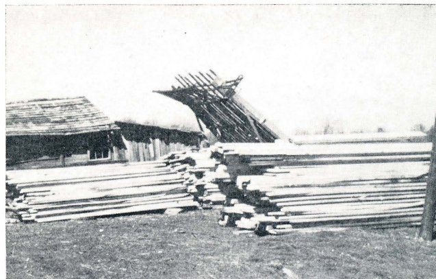
Green lumber piled in this manner will stain, warp, twist, and cup until it is not suitable for use. Much home-sawed lumber is wasted annually because of improper piling.
