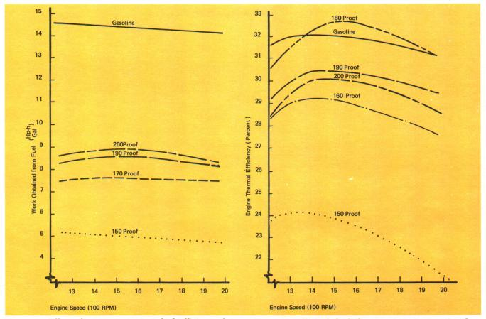
Figure 2—Effect of water content on fuel efficiency for alcohol used in a laboratory engine (5).
