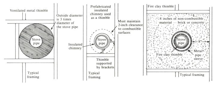
Fig. 4. Thimbles for safely passing stove pipe through combustible walls.
