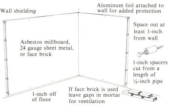
Fig. 2. By providing wall protection, you can place a wood stove closer to the wall. Leave at least a 1-inch gap between the protection material and the wall to provide ventilation.
