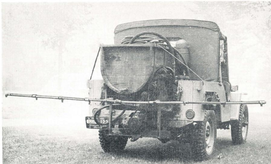
Fig. 1. A jeep-mounted power sprayer. Note the chain drive from power take-off of jeep and boom mounting. Better visibility on the part of the operator is obtained by mounting the boom in front of the vehicle.
