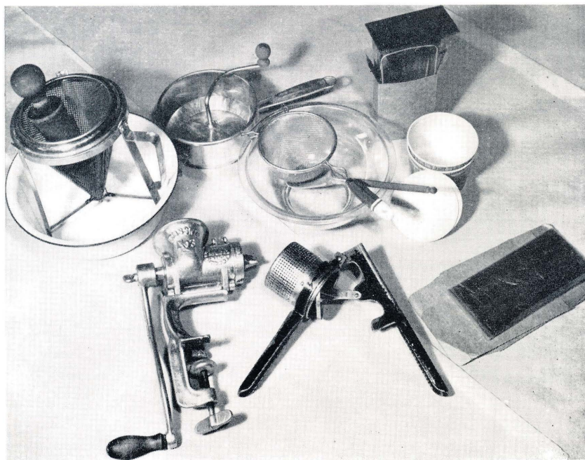
Fig. 1 — Equipment and packaging materials for preparing and packing fruit purees for freezing: (front row, left to right) food grinder, potato ricer, rectangular cartons with cellophane bag liners; (back row, left to right) conical sieve and wooden pin, Foley Food Mill, sieve and wooden spoon, rectangular carton set up showing rack and funnel for filling, heavily waxed cardboard tubs with slip-in lids.
