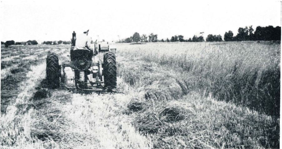
Fig. 10. The same field of bromegrass-alfalfa shown in Fig. 9. The mower with windrow attachment followed the combine around the field. Note the combine in the distance ahead of the mower.
