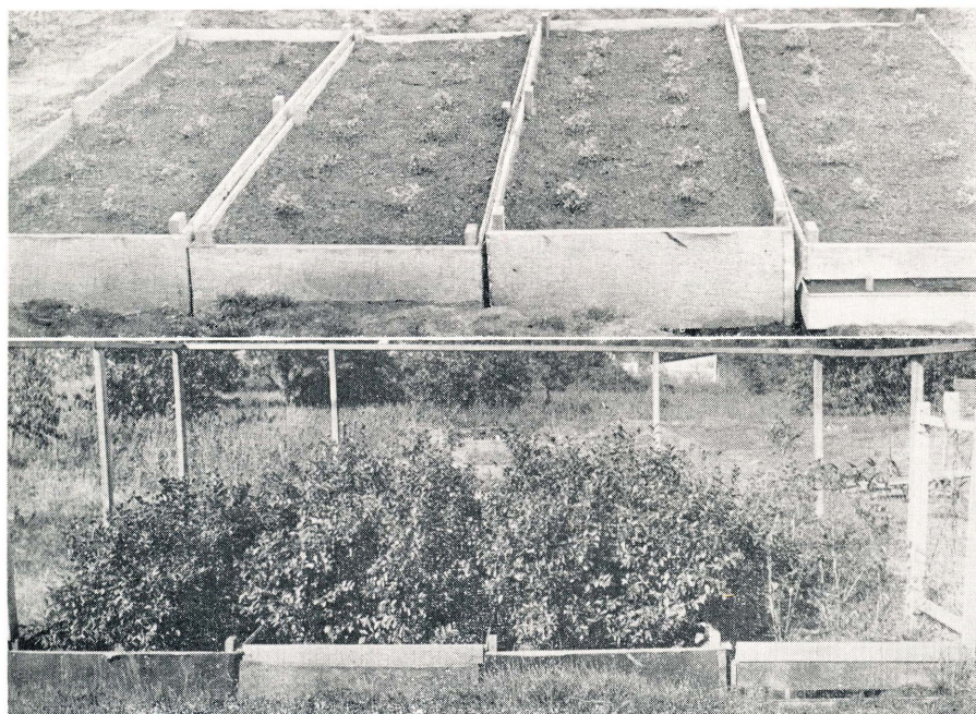
Fig. 3. Rubel plants with water table constantly maintained at different depths. Above: Plants soon after setting. Below: The same plants after 4 years' growth. From left to right: Water table maintained at 30, 22, 14, and 6 inches. The 30-inch water table did not furnish sufficient moisture, while the 6-inch water table was too near the surface.
