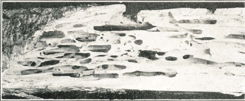
Fig. 6.—Log tunneled by large carpenter ant, reduced
