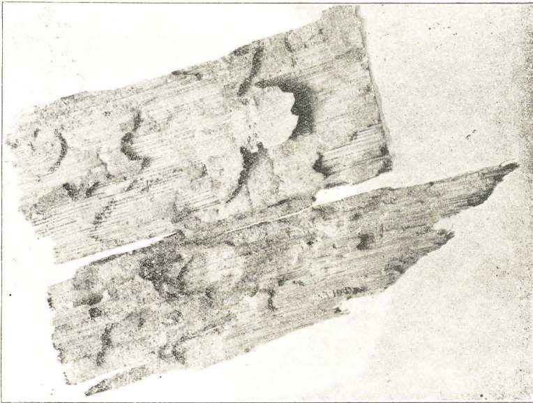
Fig. 1.—Work of termites in timber, reduced
