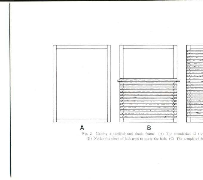
have sufficient bearing on the seedbed frame. For a 15-foot seedbed, it will be more convenient to make two shade frames each  $7\frac{1}{2}$  feet long.
