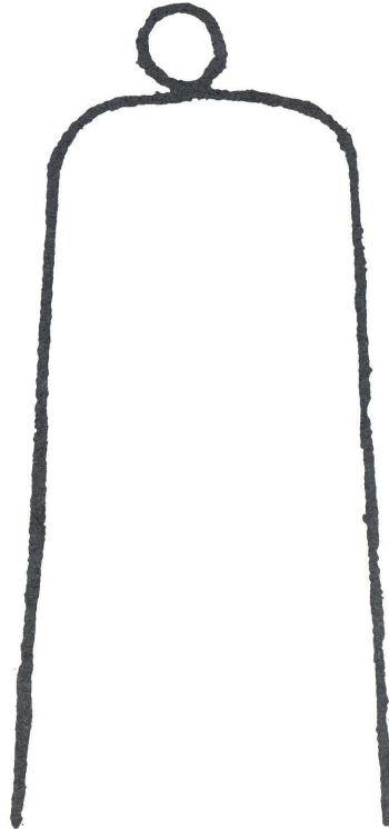
A skin shaper or stretcher can be made from a five-foot piece of No. 9 galvanized wire.
