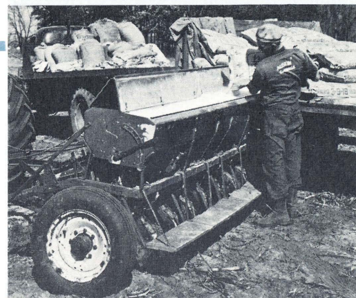
Fig. 18 Keep the fertilizer attachment cleaned out.
