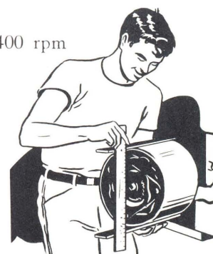
Fig. 8 Measuring a pulley.
