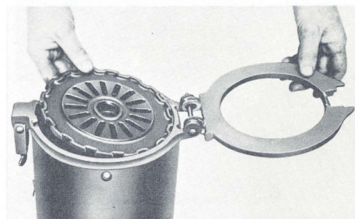
Fig. 27 Checking the seed plate on a planter.
