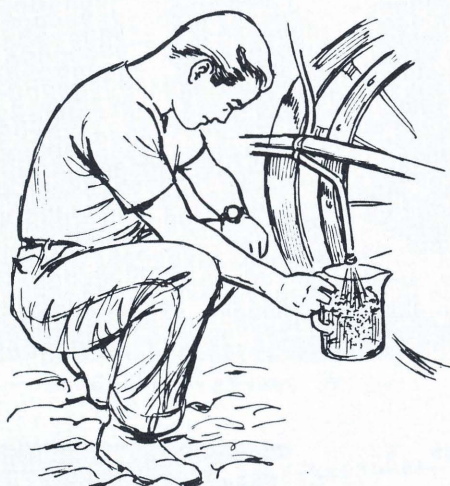
Fig. 12 Checking nozzle discharge rate.
