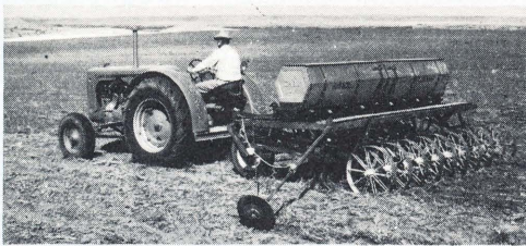
Fig. 1 A grain drill is one kind of seed planter.
