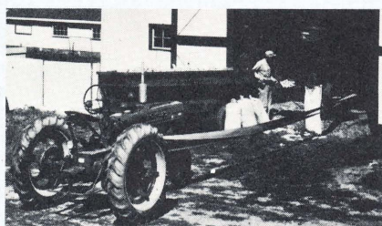
Fig. 15 Putting a twist in the belt reverses direction.
