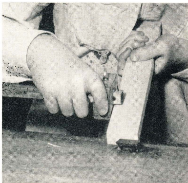
Fig. 19. Using the marking gauge.
