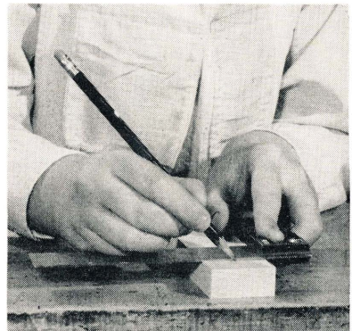
Fig. 16. Squaring the end surface.
