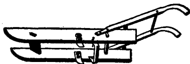
FIG. 31.— Implement used for cutting sod, also shown in operation in Plate XIII.
