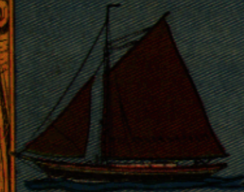
SLOOP. ONE MAST, JIB AND MAINSAIL
