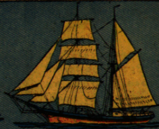
BRIGANTINE. TWO MASTS, SQUARE RIGGED ON FOREMAST ONLY. THIS IS PROPERLY A HERMAPHRODITE BRIG, BUT ALMOST UNIVERSALLY CALLED BRIGANTINE.
