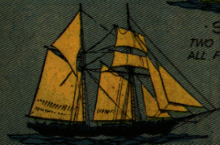
TOPSAIL SCHOONER. SQUARE TOPSAILS ON FOREMAST, FORE AND AFT ON MAINMAST.
