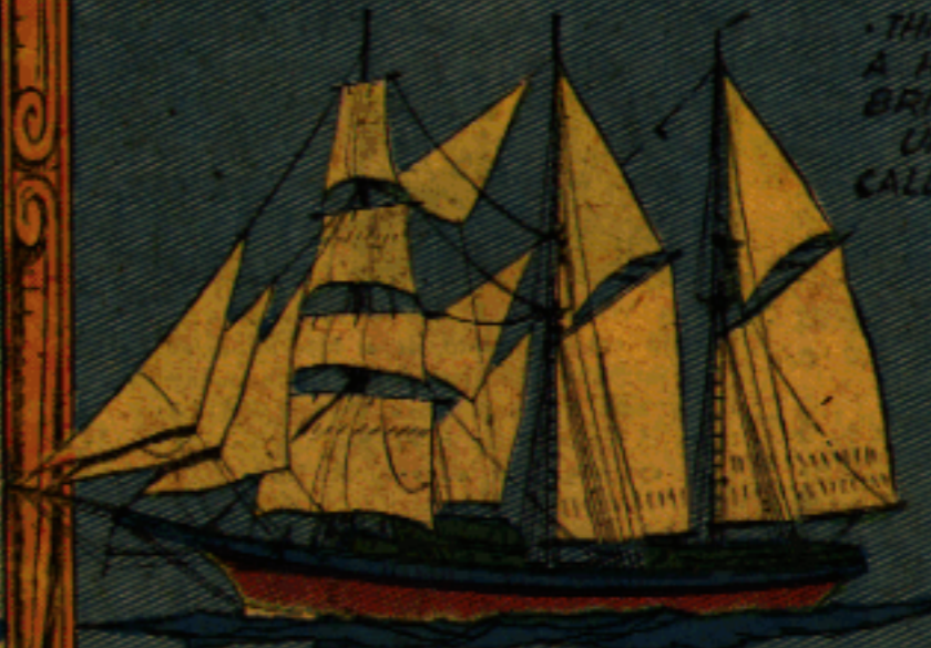
BARKENTINE THREE MASTS, SQUARE SAILS ON FOREMAST, FORE AND AFT ON MAIN AND MIZZEN MASTS.
