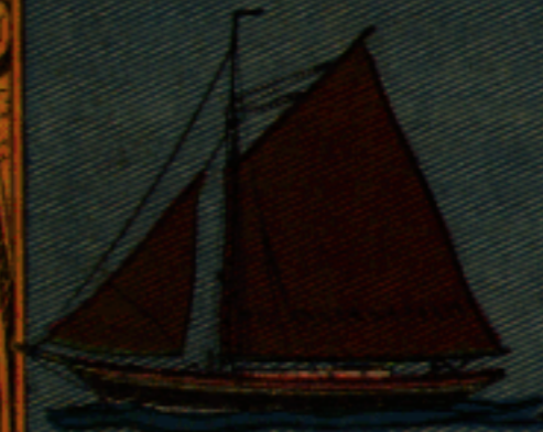
SLOOP. ONE MAST, JIB AND MAINSAIL
