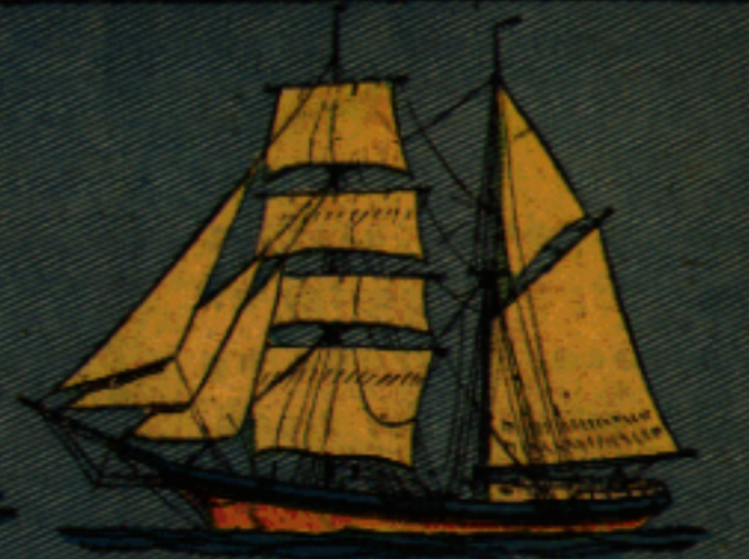
BRIGANTINE. TWO MASTS, SQUARE RIGGED ON FOREMAST ONLY. THIS IS PROPERLY A HERMAPHRODITE BRIG, BUT ALMOST UNIVERSALLY CALLED BRIGANTINE.
