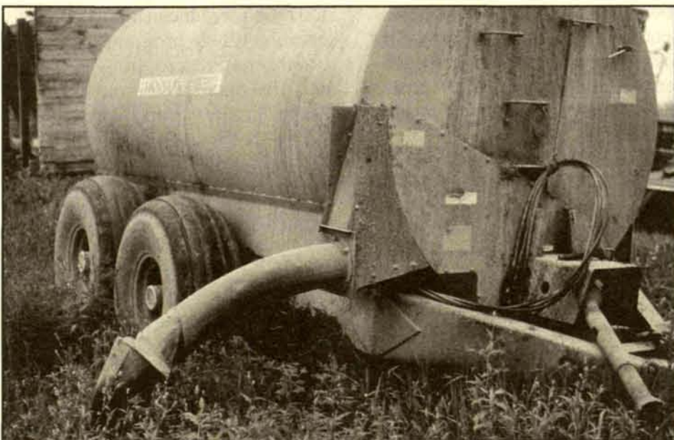
To facilitate liquid manure applications in standing corn, a special manifold was built to direct manure between the rows.
