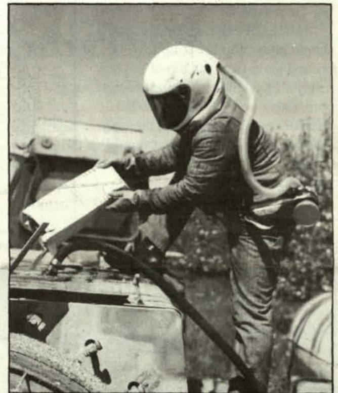
An air-purifying helmet provides the wearer complete respiratory protection from dusts, pesticides and ammonia while protecting the head and face.
