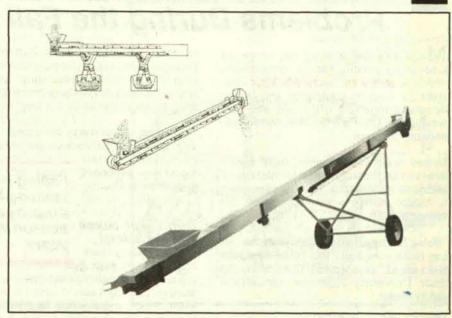
The flexible conveyors can be tailored to fit current needs and upgraded as your needs change. Equipment available includes chassis for portability, discharge spout, inlet hopper, tow-hitch, raised cover to convey higher material, and 8 foot add-on sections. For free literature or more information, contact Cardinal Grain Systems, at (219) 244-4654.
