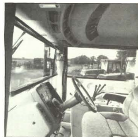
Eliminate cab window glare and reflect heat with the Designer Shade. The see through shade is mounted on a 1" metal tube and is rolled up and down on the side by a beaded chain. The bottom also has a 1" aluminum bar with suction cups for stabilization. According to the manufacturer, shades are custom made per your specifications and carry a five year warranty. For more information contact Designer Shade at 1-800-344-9090.
