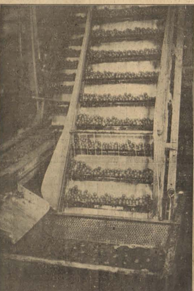
6 Three ribbons of cherries from the picking tables converge into two on separate belts taking cherries to the pitters. They are washed in running water and sprayed en route. At the top they drop on a belt, from which diversions are made for each pitter.
