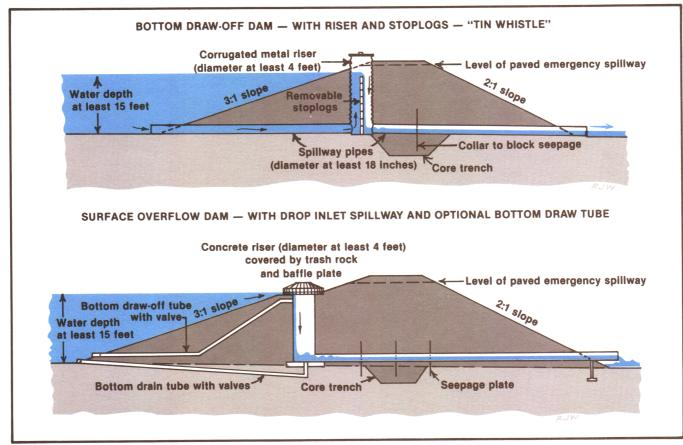
Two common types of outlet structures for dams that form fish ponds. Riser-and-stoplog construction is the simplest design that allows controlled bottom draw-off. A drop-inlet spillway can accommodate greater variation of flow. It is needed where run-off from large land area supplies the pond and where sudden high water is expected.
