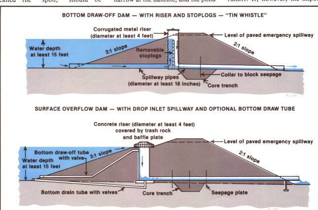
Two common types of outlet structures for dams that form fish ponds. Riser-and-stoplog construction is the simplest design the allows controlled bottom draw-off. A drop-inlet spillway can accommodate greater variation of flow. It is needed where run-o from large land area supplies the pond and where sudden high water is expected.
