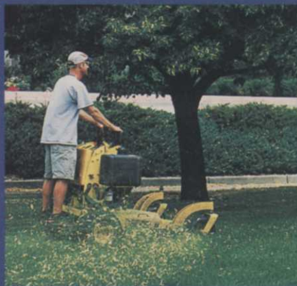
Flat ground is hard to find on Roche of Colorado Corporation's site, which is why most mowing is done with stand-on mowers.
