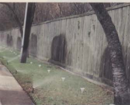
A precipitation rate test is performed on apartment property. The results are also useful to assess distribution efficiency.
