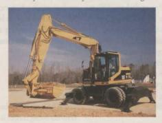
30,318 to 32,413 lbs. and is powered by a 113-hp Cat 3054 TA engine. The M315 weighs 35,082 to 36,228 lbs. and its 3054TA cranks out 114.2 hp.
