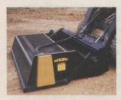
over the surface rather than turn and twist like tires. Unit has 900-lb. capacity, 65-in. lift height and is powered by a 23hp gas or diesel engine. With tracks, it's 42 in. wide.
