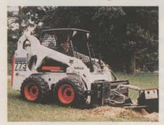
56-hp Kubota V2003T engine and increased rated operating capacity from 1,750 to 1850 lbs. New hydraulic power Bob-Tach system allows equipment changes from in the cab.
