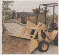
Backhoe has 92-in. digging depth with joystick controls and buckets from 8 to 24 in. Comes with 18-hp (optional 20-hp Honda) engine, hydraulic drive through a 2-speed transaxle and power steering.
