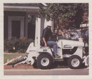
lb. digging chain rating and operating weight of 2,290 lbs. For more information contact Burkeen at 800/647-9824 or www.burkeen.com or circle no. 272.
