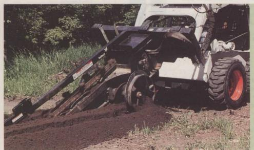
The Bobcat® LT-304 trencher attachment for skid-steer loaders can dig up to four feet deep and features a 2-in., double standard anti-back flex (ABF) chain with four different factory-installed chain and teeth options. A 14-in. adjustable auger can be removed when trenching next to fences or buildings. It comes with a manual side-shift, but a hydraulic side-shift kit is also available. For more information contact Bobcat at 701/241-8740 or www.bobcat.com or circle no. 273.
