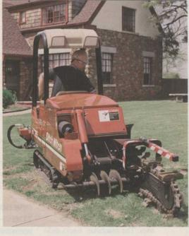
ing projects like installing sprinkler lines. Made in Perry, OK, it's just 35.5 in. wide. Unit can be equipped with a cab, backhoe, backfill blade and one of three available digging attachments: centerline, wide-centerline and offset. Optional drilling attachment allows installations under sidewalks and lanes. Unit is mounted on rubber tracks with hydrostatic ground drive and independent track controls.
