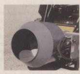
systems. Sturdy roller chain drives the drum. Ideal for mixing cement, fertilizer, potting soil or inoculating seed. It has a 5 cu. ft. capacity (one bag).
