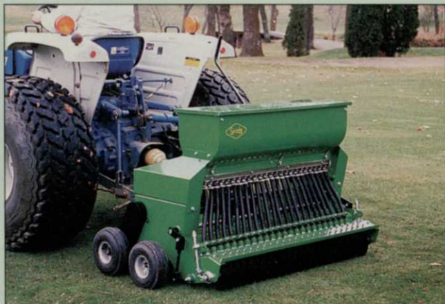
The Gandy Company overseeder holds 100-125 lbs. seed and seeds a width of 42 inches. Several Gandy models available.
