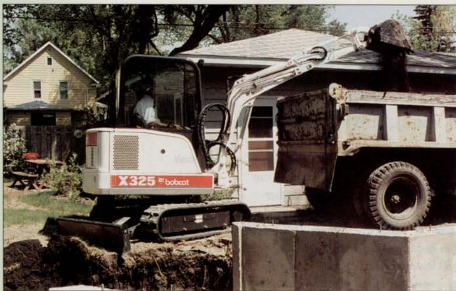
Melroe's 325 Bobcat features multi-function hydraulics system allowing simultaneous boom dipper and bucket functions.
