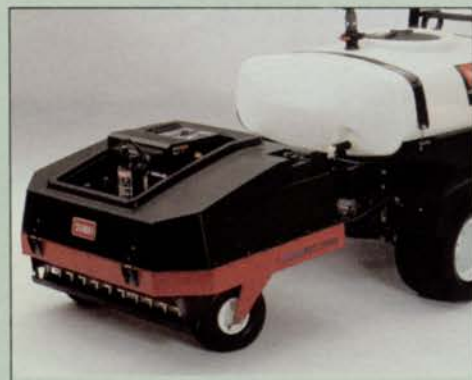
The Grasshopper Aera-vator unit is hydraulically controlled.
