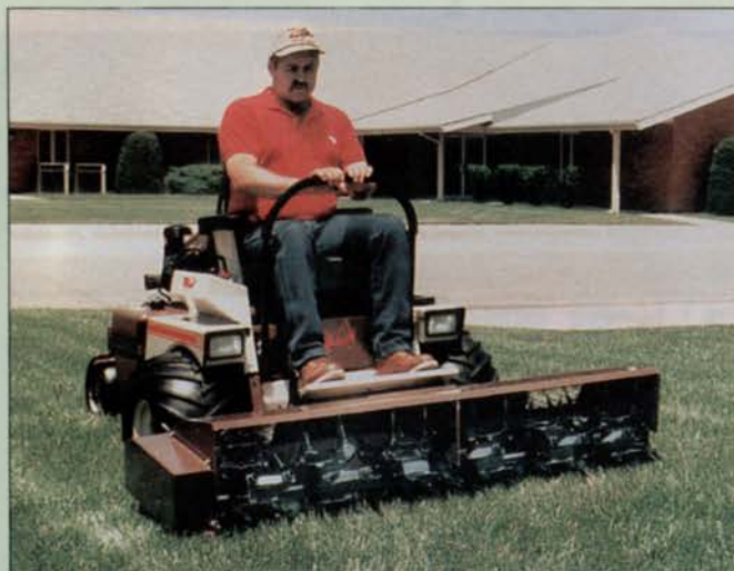
The Grasshopper Aera-vator unit is hydraulically controlled.
