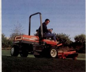
F2100 is available in 2WD or 4WD, and has 20 horsepower. Both have Kubota diesel engines, and are equipped with hydrostatic rear-wheel power steering for easy handling. A wide selection of Performance Matched Implements provide the versatility. They include triplex reel, rotary, flail and mulching rear discharge mowers, rotary broom, leaf blower, snowblower, and front blade. Roomy operator's deck, tilt steering wheel, and excellent visibility increase comfort and productivity.
