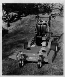
Single-adjust caster pins allow quick adjustments in mowing heights from 11/4 to 5 inches in 1/4-inch incre-
