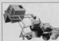
MODEL 70-LD Sweeps 54" wide. Self-propelled. 2 cu. yd. ground dump hopper.
