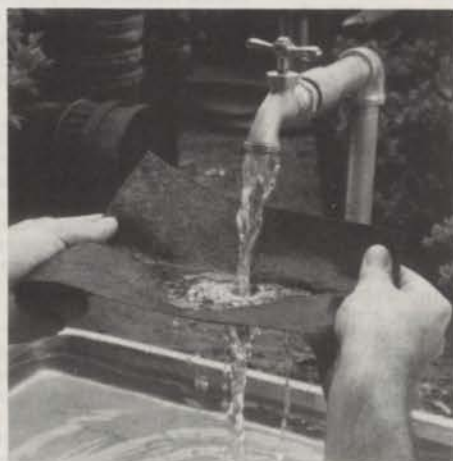
Water passes easily through highly permeable Duon Weed Control Mat.
