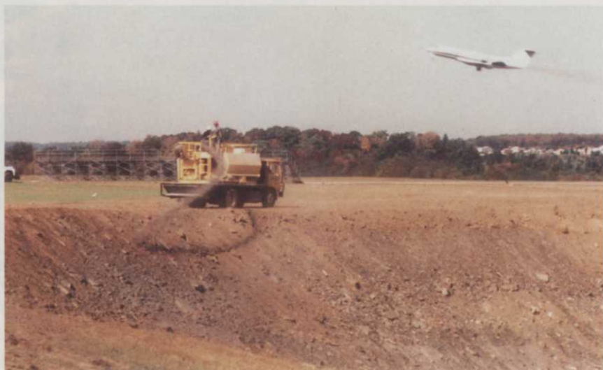
The Reinco Hydrograsser uses hydro-jet agitation with a grinder/blender feature.
