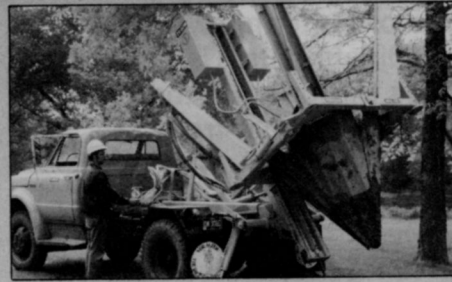
TS-50M. Truck-mounted. Outstanding maneuverability. Extension and side-shift features let you hydraulically position the spade an additional 21" away from the frame and 15½" left or right of center.
