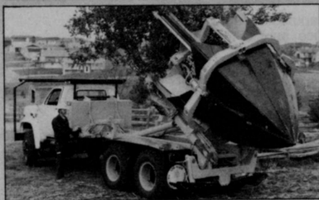
TS-84T. Truck-mounted. Transplants trees with maximum trunk diameter of 8". Six hydraulically activated, high tensile steel spades. Gravity-feed water tanks for spade lubrication.
