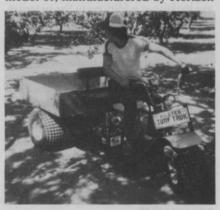
Services Company, features a twopassenger bench seat, electric start G300 Honda industrial engine, 3 ft. by 4 ft. cargo box and a load carrying capacity of 1200 lbs.
