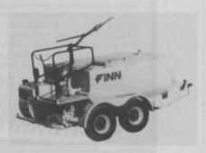
Finn Corp.'s T80 tank features a low profile tank design for ground level loading and a hydraulic powered, variable speed paddle agitator.
