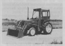
tractor. The Custom 300 cabs are ROPS-tested to meet OSHA requirements and feature all-steel construction, tinted safety glass, sliding rear window and vinyl padded interior.
