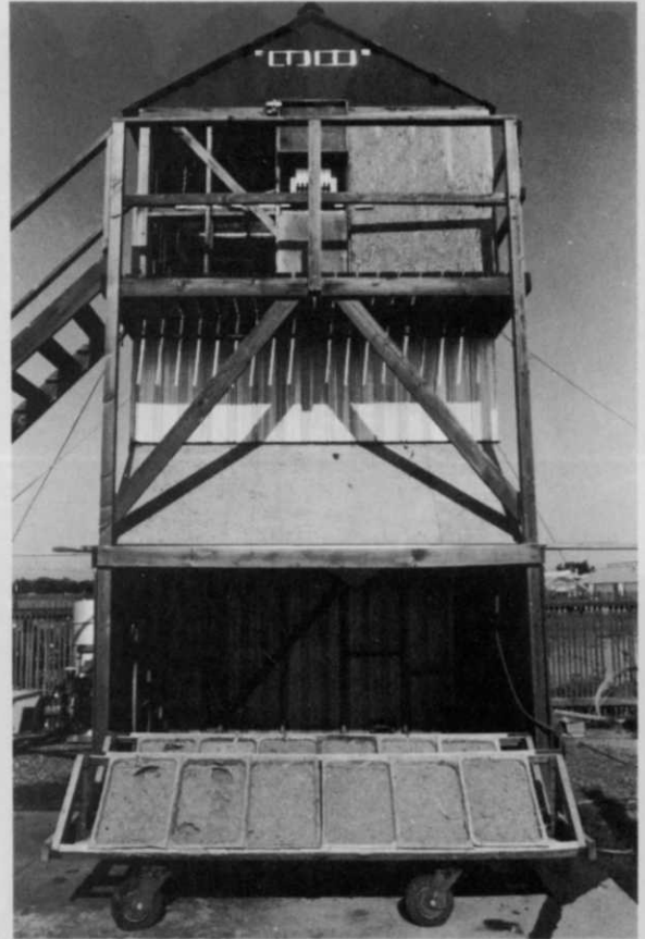
Figure 1 (above): Raintower produces artificial rain which strikes the surface of erosion-control treatments on inclined surfaces.
