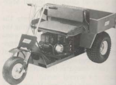
POWER-KART from Snow Company will haul up to 500 pounds gross at speeds of up to 20 mph. It's powered by an 8 hp engine and has a variable speed drive. Low bar rear tires are standard. Knobby tires, shown, are also available.
