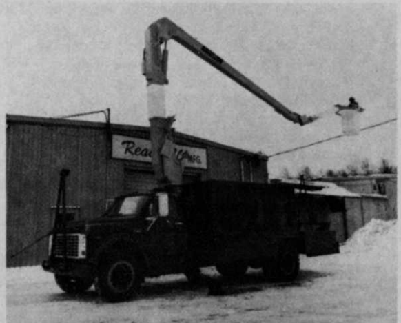
REACH-ALL increases your working area with its modern 3 knuckle design and includes fiberglass lower boom insert.
