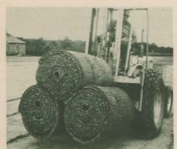
Harvest, load, and lay sod FAST, without manual lifting or handling. Let tractors do the hard work. Hand stacking and laying of sod is obsolete. Increases sales by cutting time and cost of installation. Stretches sod 3% to 5%, leaves lawns smoother, with fewer seams and joints. Disposable cardboard tubes are lighter and cheaper than pallets, permit easy loading, as many as 3 rolls at a time, with any fork lift, laying with any tractor.
