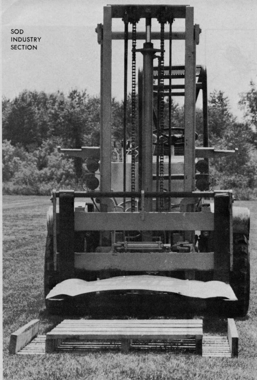
A Baker-York towable lift and disposal cardboard pallets are the cost-cutting keys to a Michigan sod producer's delivery system. The wood pallet is specially designed for use with cardboard.
